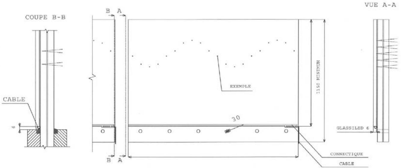
**Figure 16 – Verre complet Balustra L Glassiled et câblage**
